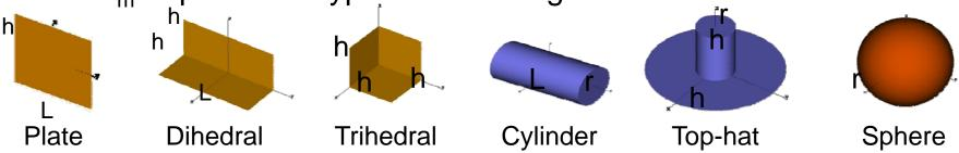
Rigling's (SPIE 2004) bistatic parametric scattering models modified to account for object radius and amplitude scaling to radar cross section
