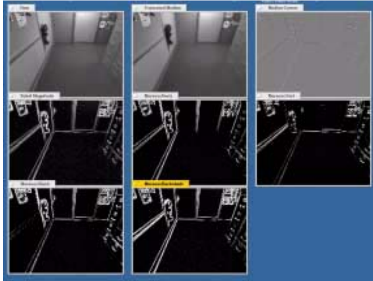
Figure 2: A dewarped image and the image operators applied to it: truncated median, median corner, Sobel magnitude, and four directional Moravec interest operators.
