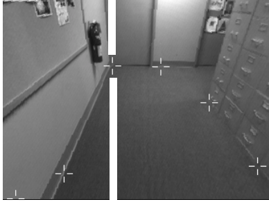
Figure 3: What is computed. For a given column of the image, the evolved vision subsystems compute the boundary between the ground (lower line) and a non-ground object (upper line). If there is more than one such boundary, the lowest is desired. This is done independently for six columns in the image.
