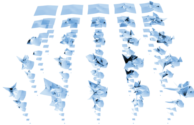
Fig. 3. Butterfly Machines Project: Fuchs used Genr8 to assemble multiple families of Genr8 surfaces that were self-intersecting. Each family is a simple parametric variation of the square rewrite system. Across families, the location of attractors and repellers varies. Placement was chosen to promote the chance of self-intersection during growth. Within a family, different surfaces are generated by experimenting with the strengths of attractors and repellers at fixed locations. This image captures one family both in time, and, in repeller and attractor space. Each surface ‘grows’ along the vertical (time) axis. A vertical slice of the 3 dimensional projection shows the family’s surfaces responding to different attractor and repeller strengths at a (time) step in the development.
