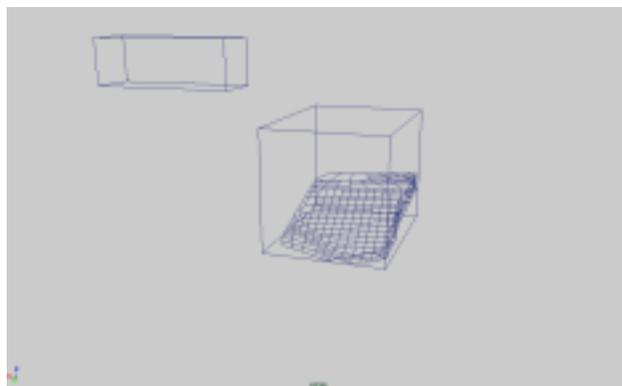
Figure 5: Surface inside a bounding box. The repeller in the upper left corner pushes the surface into the corner of the bounding box.
