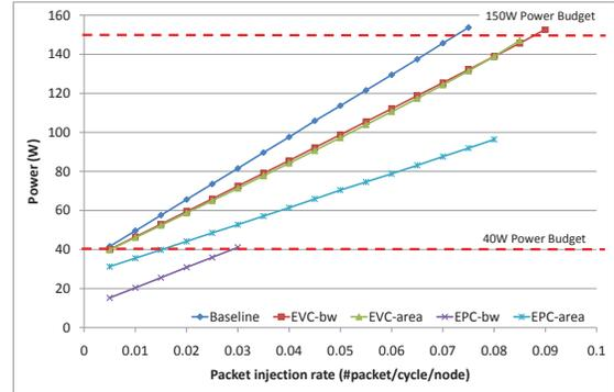
Fig. 6. Power-Performance Curve with Normal Cu Wires
