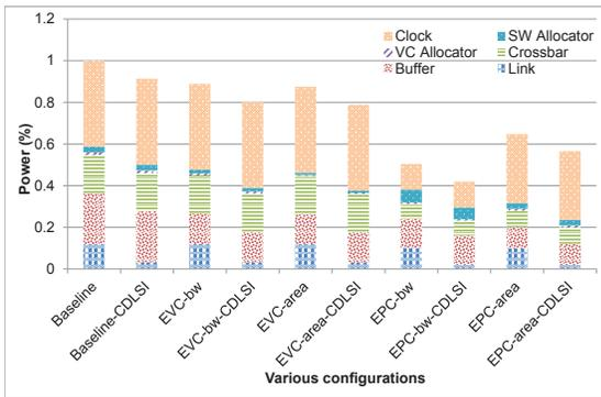
Fig. 9. Network power breakdown for various topologies
