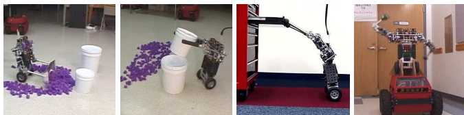
Fig. 1. The uBot-4 performing plowing, stacking, pushing, and throwing tasks.
