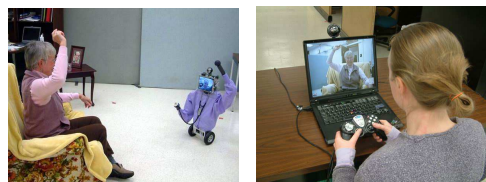
Fig. 2. A three-question stroke diagnosis through video phone with motor tasks that are demonstrated by the uBot.
