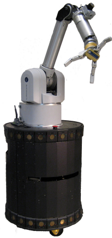
Fig. 2. UMan (UMass Mobile Manipulator)
